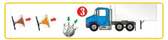
Apply both the tractor and trailer parking brakes using the appropriate airbrake system controls (the trailer supply valve [red knob] and the spring brake control valve [yellow knob]).
