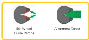
Confirm that the kingpin is aligned so that it will only contact the guide ramps of the 5th wheel lower coupler. Adjust height if necessary so that contact of the upper coupler will be on the bottom half of the 5th wheel lower coupler face.
