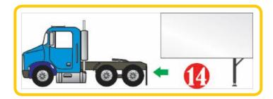
**NOTE:** For a tractor with an air suspension drop feature, raise the tractor suspension to the normal position.
