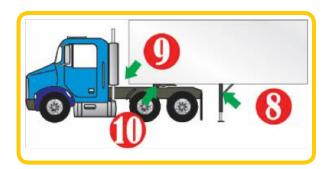
**Note:** In some cases, the trailer suspension will drop when the air is exhausted out of the supply line. This can cause the trailer to shift a little forward or backward. This movement can cause the 5th wheel to jam, making it impossible to pull the 5th wheel release handle. When this occurs, you can reverse the tractor a little, to relieve the tension. Sometimes
