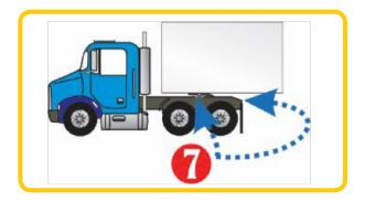
Get into a position under the trailer to visually check that the 5th wheel locking mechanism is in the proper closed position. Watch your head as you get under the trailer and wear protective head gear if that is a workplace requirement. Look for closed jaws or the lock bar position, depending on the style of 5th wheel.
