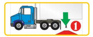
It is important that you know the approximate weight of the trailer you are towing. This will allow you to make the right decision about where you can drop the trailer. Select a location that is known to be suitable and firm enough to support the weight of the trailer.
