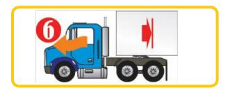
If the 5th wheel is not fully engaged and locked, the 5th wheel will release and tractor will move forward. This will require reversing again to properly engage and lock the 5th wheel. Gently but firmly engage the 5th wheel. Listen for and feel the 5th wheel latching into its locked position.
